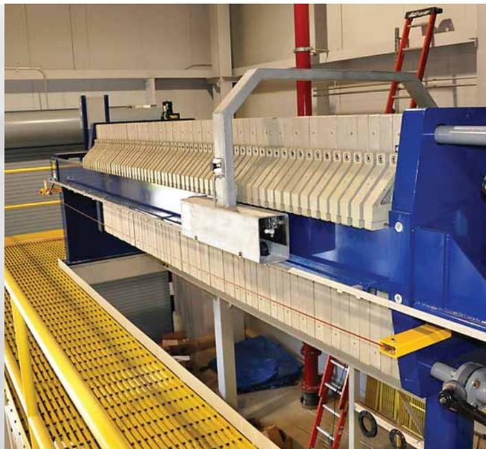
“ENGINEERED FOR PERFORMANCE IN A VARIETY OF INDUSTRIAL AND MUNICIPAL APPLICATIONS, THE FP-SERIES FILTER PRESS COMPACTS LIQUID SLURRY INTO A DRY FILTER CAKE THAT CAN BE ECONOMICALLY DISPOSED AT A LANDFILL.”
